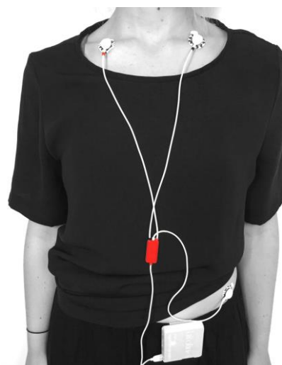
Fig. 4. Example of an assembled ECG placement with IN+ & IN- on the collarbones and REF on the iliac crest.
