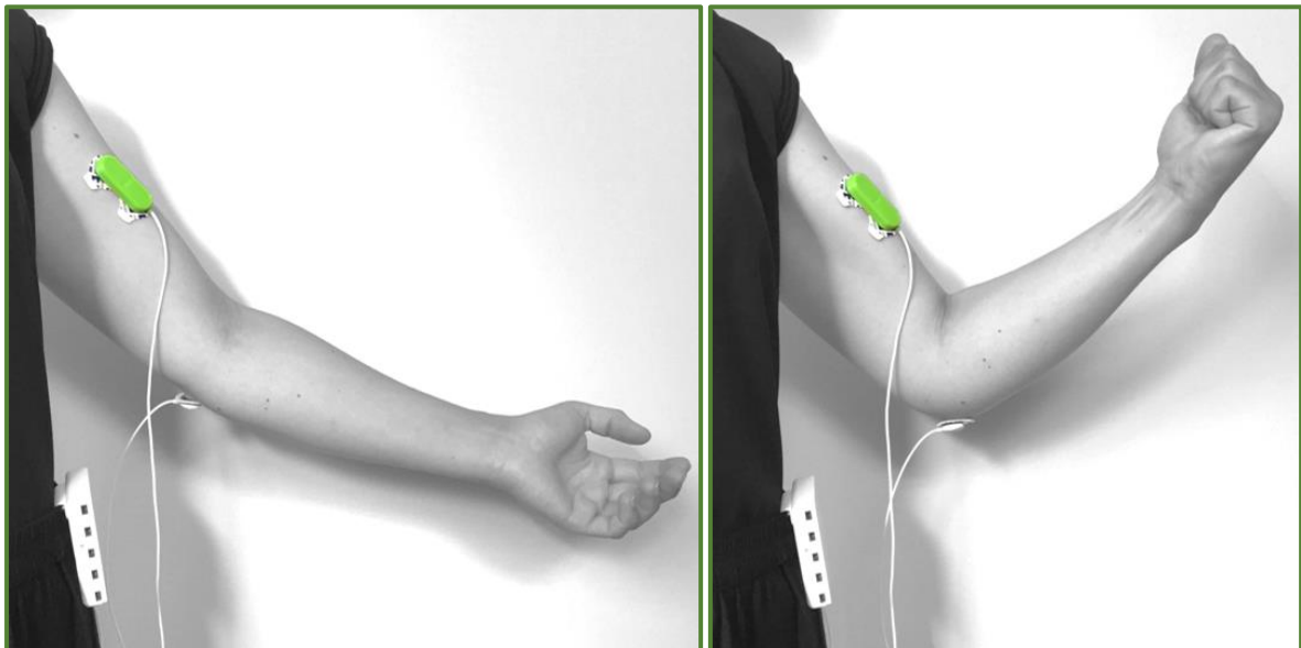
Figure 6: Data acquisition and sensor placement with the assembled BITalino EMG sensor on the muscle biceps brachii.
