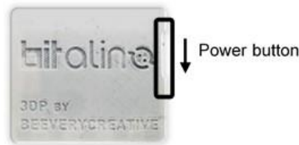
Figure 2: BITalino (r)evolution Assembled Core BT: Power button location on the right side of the device.
