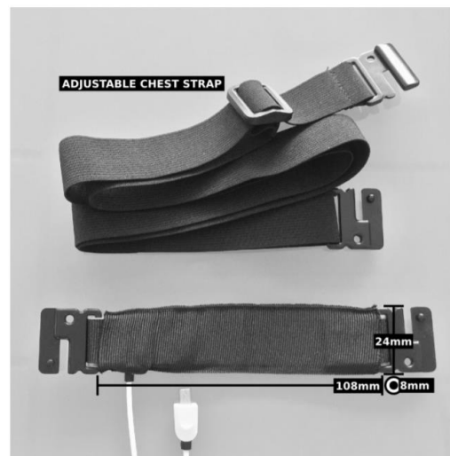
Fig. 1. The sensor is provided with a convenient elastic chest strap to secure it in place.
